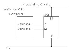
(\*) MVE contain a half-wave rectifier power supply. They must not be powered with transformers that are used to power other devices using not isolated full-wave rectifier power supply.
