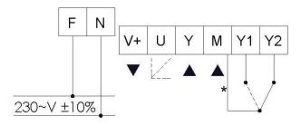
\* Floating only sink connection (connect Y1, Y2 to M).
